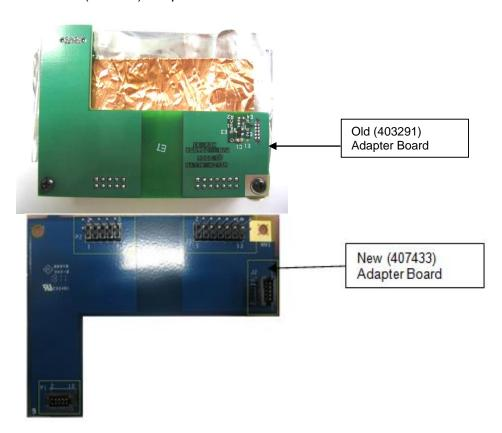
4. Unwrap the EMI shield from the SpO2 Module. Note the difference between the old (MS-11) and the new (MS-2011) modules.
