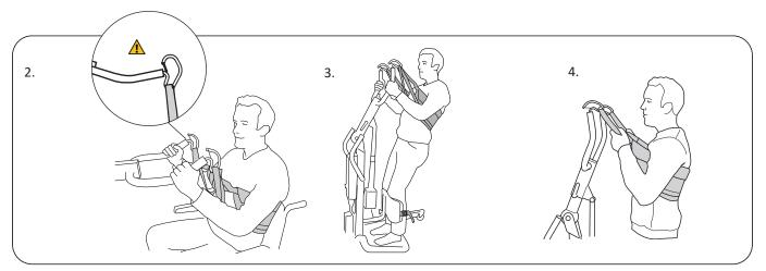
2. Roll the Sabina<sup>™</sup> lift towards the patient. Adjust the base width so that the lift comes close enough to the patient. The patient's feet are to be placed on the centre of the footrest. Adjust the depth of the lower leg support so that the patient's shins are parallel with the support. Adjust the height of the support so that the upper edge is just beneath the kneecaps. Fasten and tighten the calf strap.
